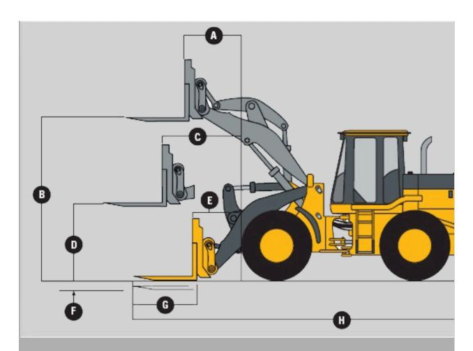
**Dimensions** (with Quick-Coupler and Construction Fork)
